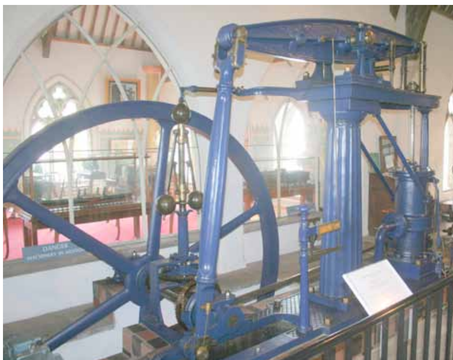
The single-pillar beam engine acquired for the Smithwick brewery in Kilkenny in 1847. Cylinder 12in x 27in; flywheel 10ft 6in diameter; beam length 8ft 6in.
