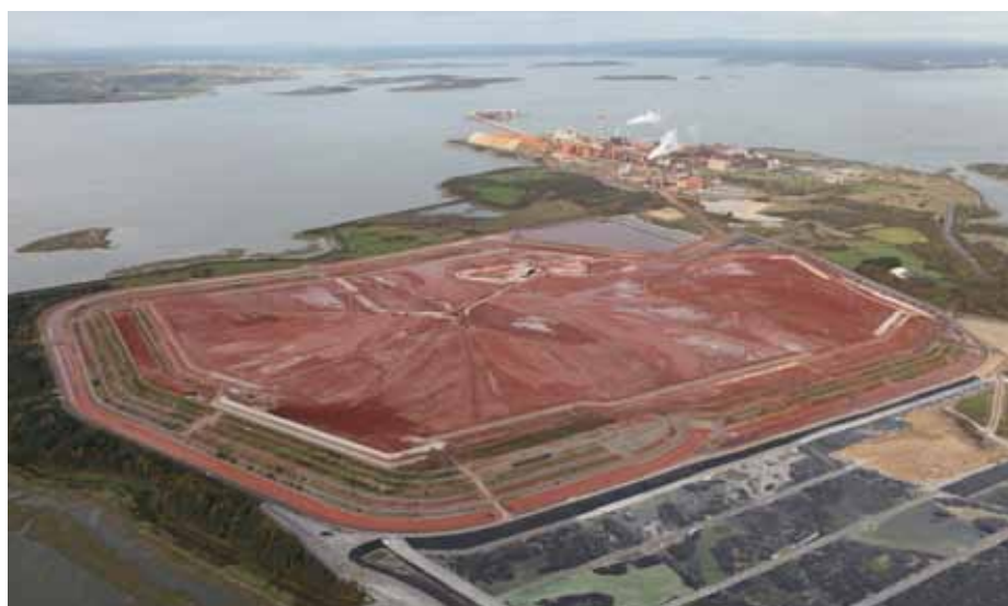
An aerial view of the Aughinish Alumina site with the bauxite residue, or red mud in the foreground and the kilometre long quay for the berthing of ships of up to 60,000 tonnes in the distance. Photograph © Brady Shipman Martin
