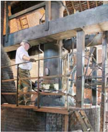
The Engine now operates automatically but requires supervision as the valve mechanisms occasionally fail to trip, usually due to inevitable slight variations in the supply of steam.
