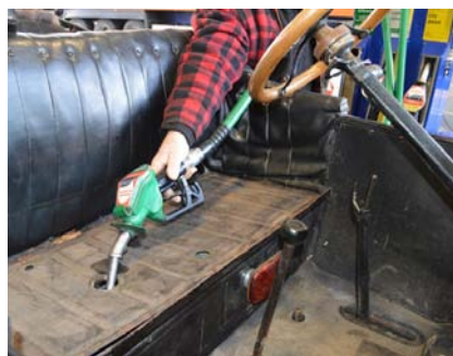
The petrol tank is beneath the seat.
