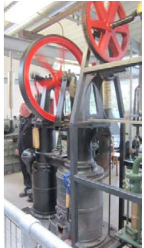
A Hayward-Tyler Ltd, 1880 Hot air engine (1 hp)
