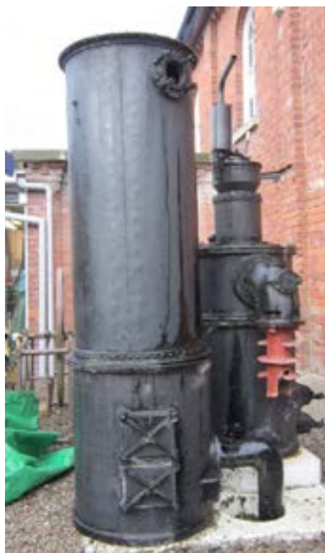
National gas producer plant (gas scrubber and retort). No date but about 1920
