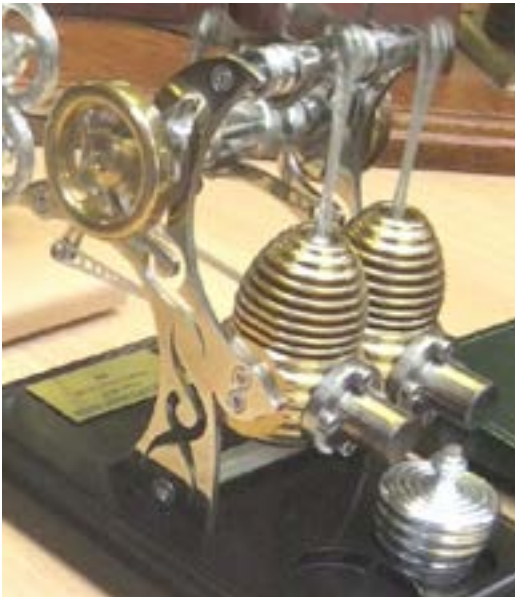
A Bohm Two Cylinder Stirling. A spirit burner is in the right hand corner
