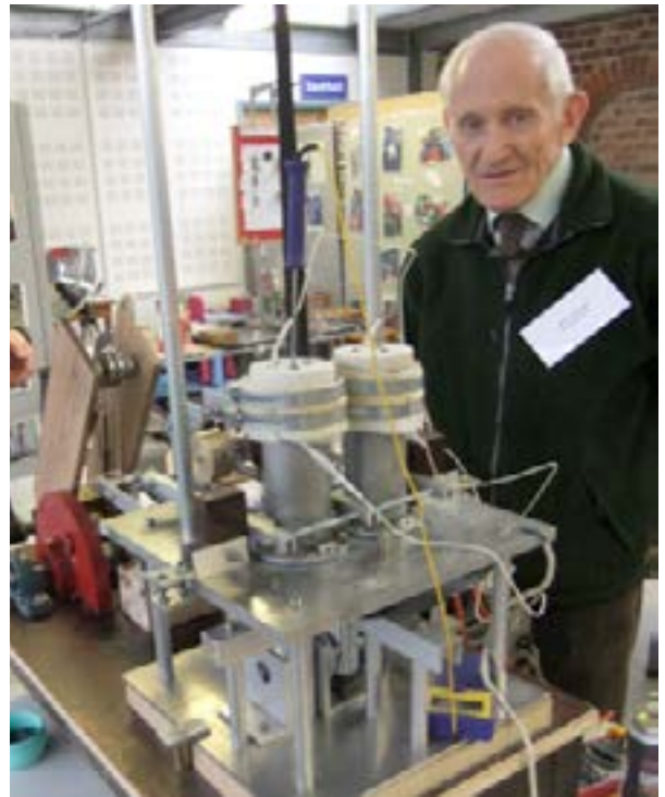
Austyn Williams stands beside his novel Stirling Engine in which the two displacer cylinders are prominent on the upper part of the machine
