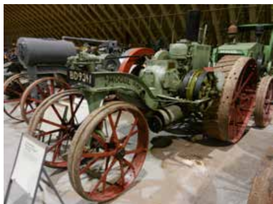
An International Harvester Mogul 8-16 c1914 which was used in Norfolk. The narrow front axle provides clearance for the belt drive and reduces the turning circle of the tractor.
