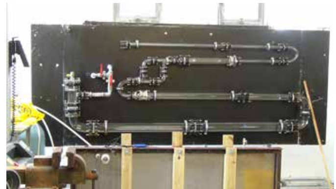
Rig to demonstrate how crushed ice can be used for cleaning pipework
