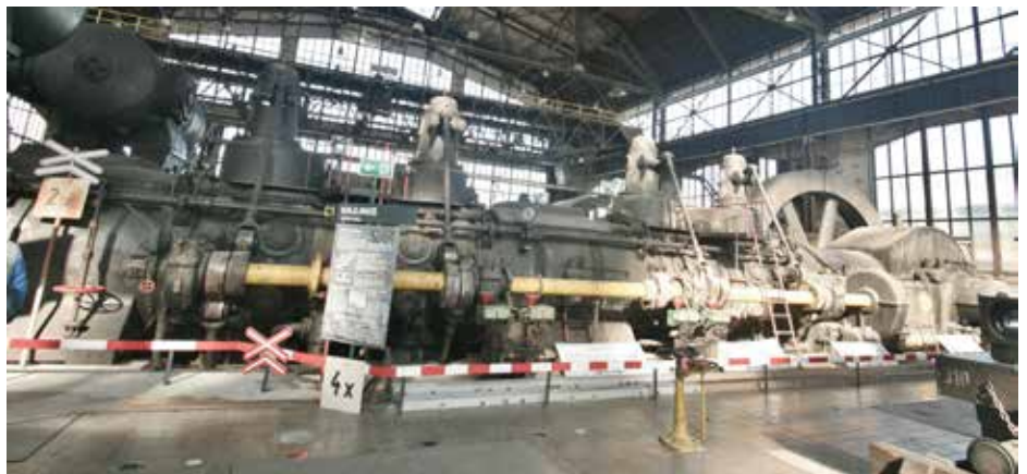
The 900 tonne gas-driven blower at the Vitkovice steelworks, made locally in 1938. It ran at 80 RPM and developed 3800KW
