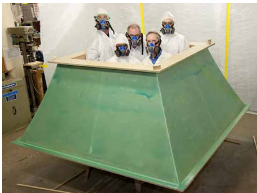
Science Museum Workshops staff pose for the camera inside the largest of the six moulds they made. Left to right: Kevin Carlin, Jake Fuller, Chris Ward, Frank Lincoln and Mike Ashelford. The mould is seen with a wax coating, a gell coat and finally chopped strand matting with resin. Image: D131570 © Science Museum / Science & Society Picture Library -- All rights reserved.
