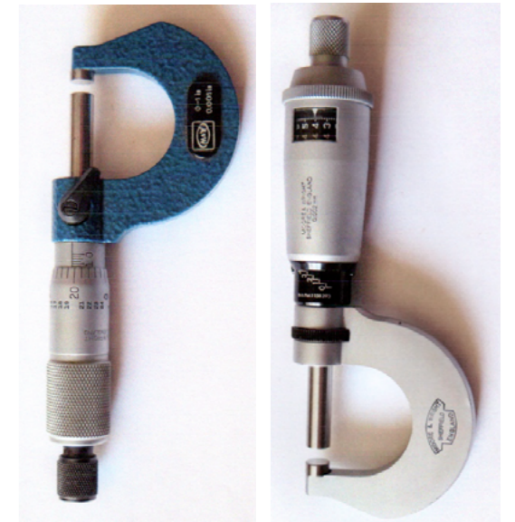
Left: Braille micrometer, a micrometer for left handed inspectors. Right: A 1969 direct reading micrometer
