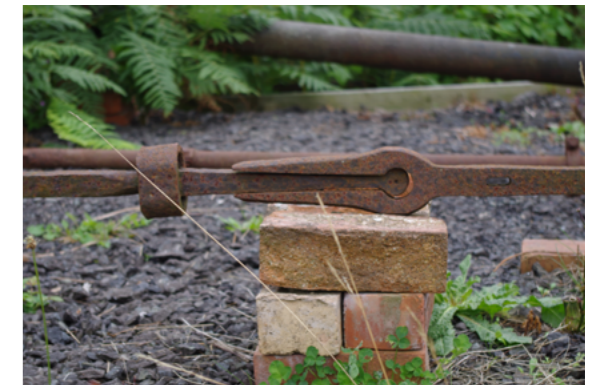
Salt works are basic engineering. A simple fail-safe connector in the pump rods at Lion Salt Works.
