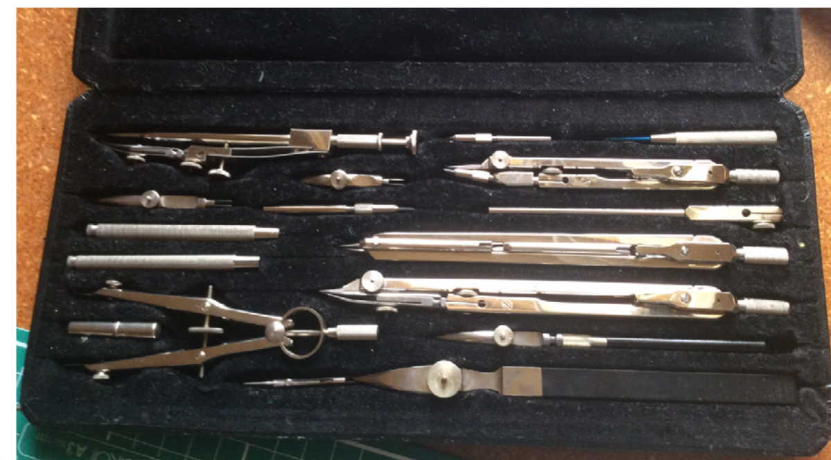
Case of drawing instruments (German-made ‘Precision’). The drop compass is top left.
