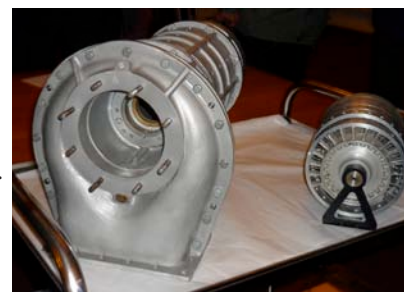
Exhibits from the Science Museum Collection. Top:- A A Griffith's compressor-turbine test rig, 1929 (Inv 1983-231)
