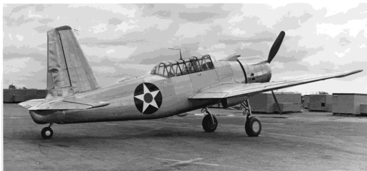
Figure 3. The ram air induction scoop above the cowl, fitted to the V-85, is shown to good advantage in this shot. The metallized rudder (as opposed to the standard fabric covered version) helped the aircraft to handle 3,000 plus horsepower. (Pratt & Whitney Archives)
