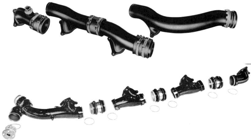
Figure 14. Two styles of intake manifold design. Early, “hose clamp” type at top and later chevron seal type at bottom.
