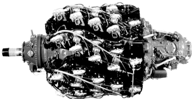
Figure 4. The R-4360-25 was the production version of the R-4360-5. This typifies a mid-production R-4360. Note the six-inch extension incorporated into the nose case – a feature of all B-36 engines. This extension accommodated the propeller spinner afterbody.
