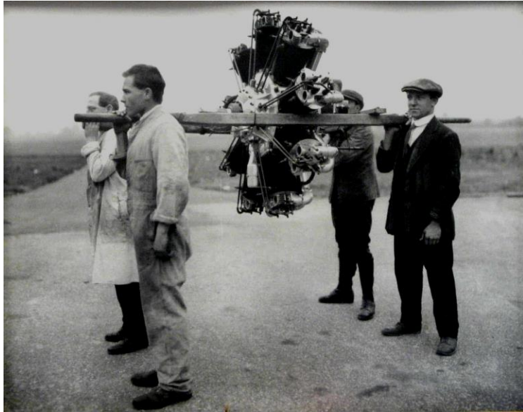
Figure 4 The Brazil Straker or Cosmos Jupiter which became the basis of a long line of radial engines from Bristol.
