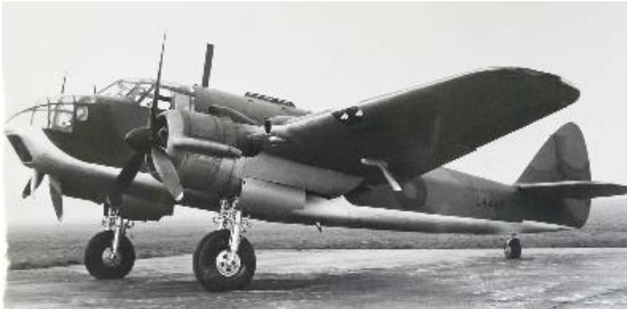
Figure 13. The Bristol Beaufort torpedo bomber. Engine failures of the Taurus in this aircraft lead to the maneton clamp having to be redesigned.
