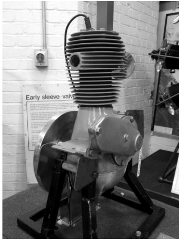
Figure 5 The Barr and Stroud sleeve valve motor cycle engine.
