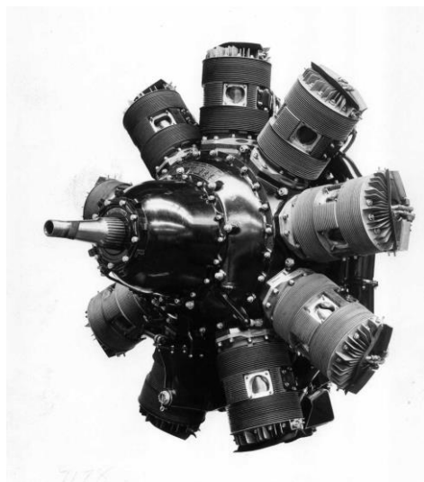
Figure 7 The Bristol Perseus. The first successful sleeve valve radial.
