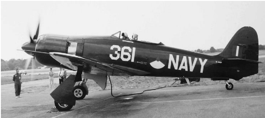
Figure 22. The Hawker Sea Fury, in which a five bladed prop is needed to absorb 2730 shp.
